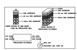
**DETAILS OF RAIN WATER HARVESTING STRUCTURES**
